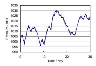
A barometric pressure measurement is an example of an absolute pressure measurement. This means a barometer would read zero when measuring a vacuum (zero pressure absolute). Most pressure instruments, such as a car tyre gauge, measure gauge pressures, so read zero when open to the atmosphere.
