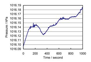
In practice, the short-term fluctuations in the atmospheric pressure are small. The graph above is the measured atmospheric pressure in a laboratory recorded over 15 minutes. It shows a variation of about 0.1 hPa due to the weather pattern and some short-term fluctuations of  $\sim 0.01$  hPa due to drafts caused by the opening and closing of doors etc.
